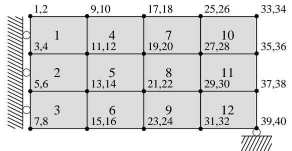
Fig. 2 The design domain with 12 elements.
