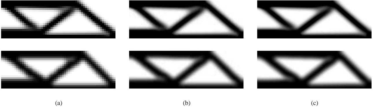
**Fig. 3** Optimized design of the MBB beam obtained with the 88 line code using sensitivity filtering (top) and density filtering (bottom). A mesh with (a)  $60 \times 20$  elements, (b)  $150 \times 50$  elements, and (c)  $300 \times 100$  elements has been used.
