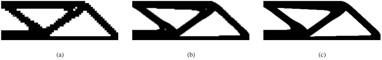
**Fig. 5** Optimized design of the MBB beam obtained with the 88 line code extended by a Heaviside filter. A mesh with (a)  $60 \times 20$  elements, (b)  $150 \times 50$  elements, and (c)  $300 \times 100$  elements has been used.
