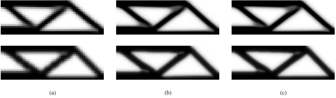
**Fig. 4** Optimized design of the MBB beam obtained with the variant of the 88 line code using PDE based sensitivity filtering (top) and density filtering (bottom). A mesh with (a)  $60 \times 20$  elements, (b)  $150 \times 50$  elements, and (c)  $300 \times 100$  elements has been used.
