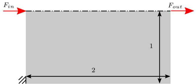
Fig. 27 Auxiliary compliance problem for the force inverter. Both forces are set to F = 1 .
