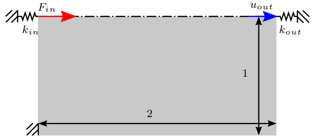
Fig. 26 Force inverter design problem. The material has stiffness E = 1 and \nu = 0.3 and the input and output springs are set to k = 0.1 . The input force is set to F = 1 .
